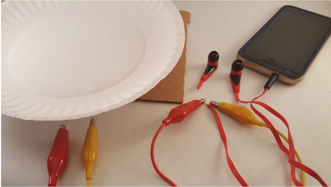
A smart phone connected to pair of headphones connected to a paper speaker.
