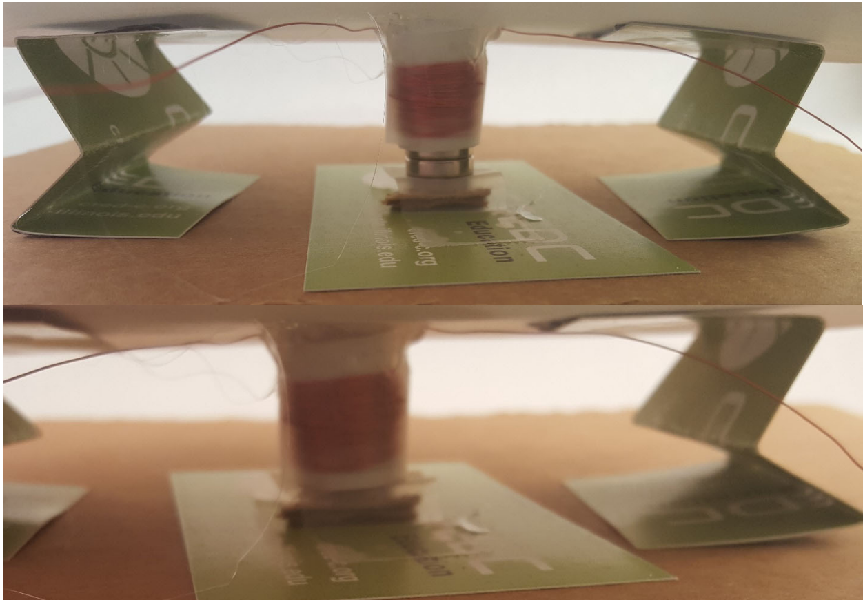
Two pictures of how the finished voice coil and diaphragm should be connected to the cardboard base and permanent magnets.
