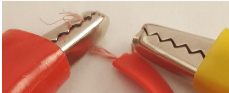
Alligator clips attached to the signal and ground wires from a stripped pair of headphones
