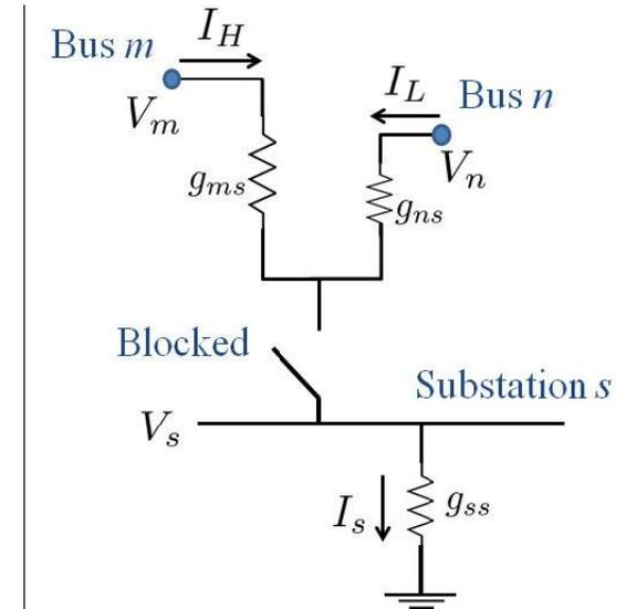
**Example:** GBD modeling at a conventional transformer located in Substation  $s$ , with HV Bus  $m$  and LV Bus  $n$
